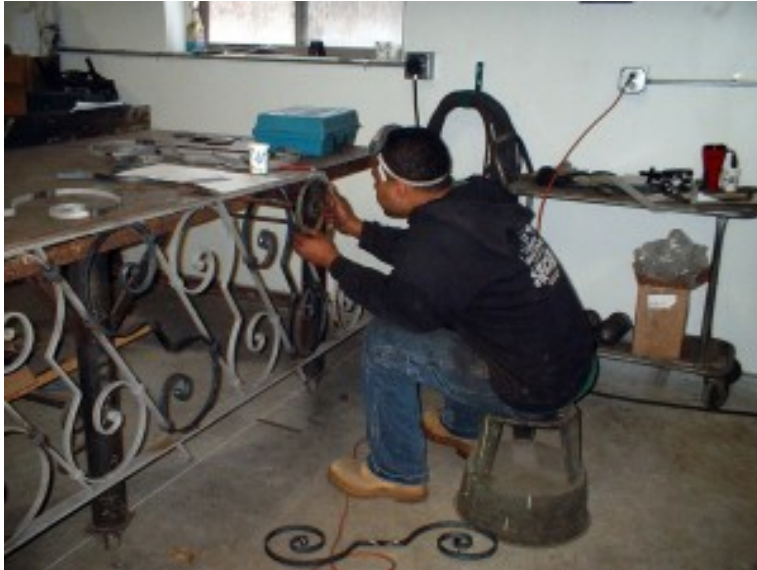
Sherwin putting a Railing together that was a restoration job.
